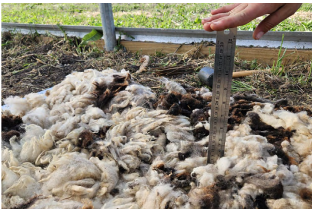
Figure 2. Raw wool was installed in a layer three inches deep.
