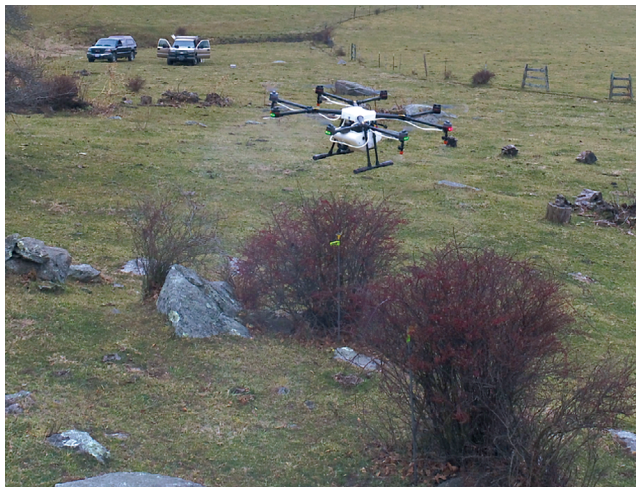
Figure 1. A spray drone being deployed to treat weeds growing in rugged terrain that is not easily accessible with large machinery. Photo courtesy of Dr. Andrew Howell, North Carolina State University
