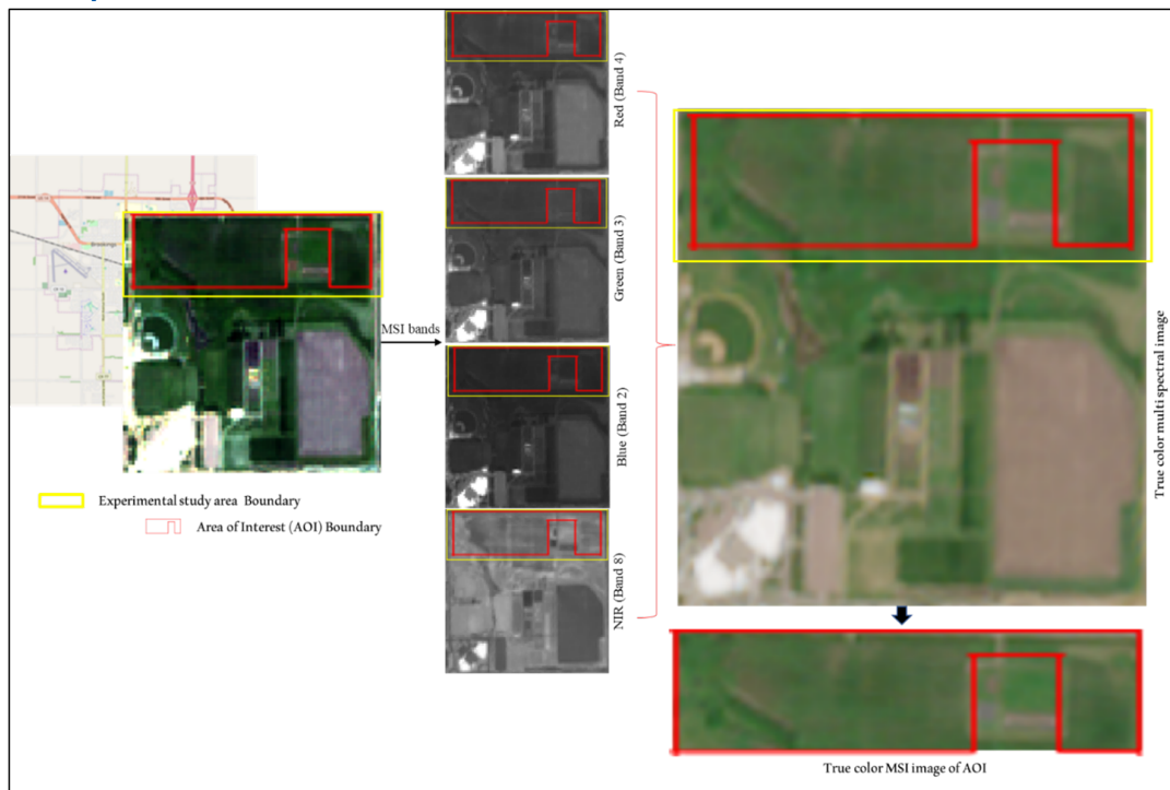
Figure 9. Example to show the results of how Sentinel-2 MSI bands (Red, Green, Blue, NIR, and Red Edge) are combined to generate a true color or false color composite image for vegetation and land surface analysis.
