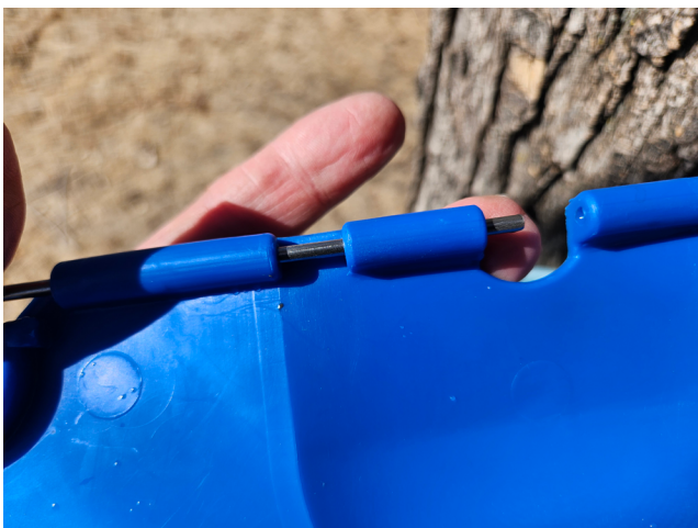
Figure 14. Removing lid rod from center slot.
