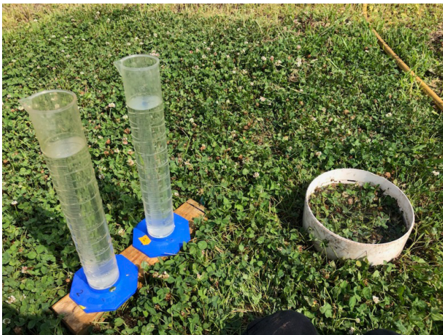
Figure 5. Water infiltration ring and two 1000 mL graduated cylinders that are used to refill it every minute.
