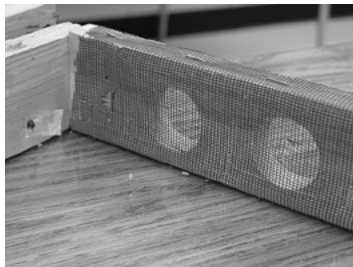
Figure 1. Holes for air flow.
