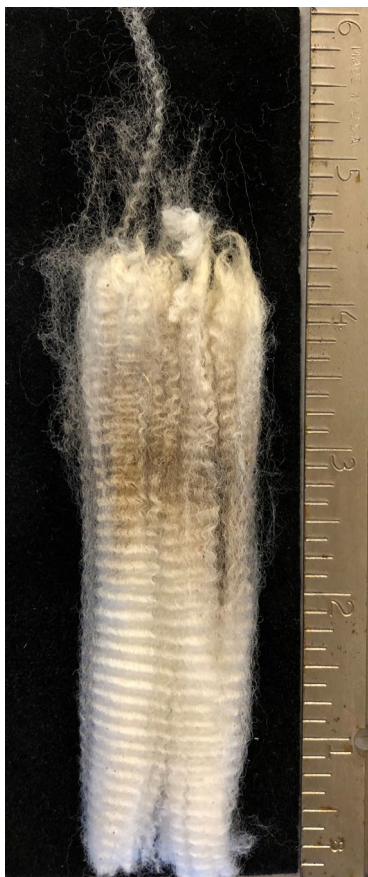
Figure 2. Example of 4.5” staple with distinct crimp design.
