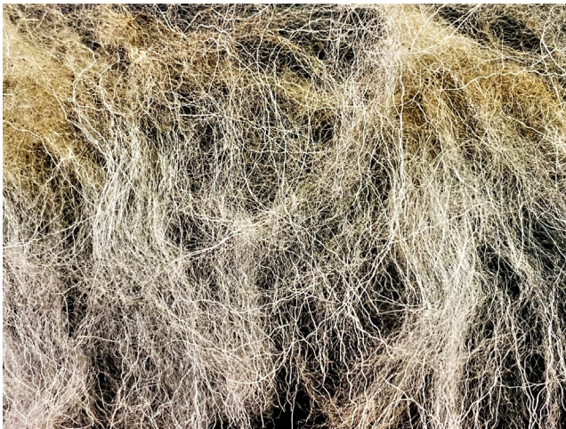
Figure 3. A sample of wool contaminated with medullated fibers (bright, white, ridged fibers).
