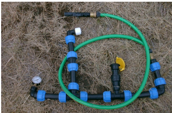
Figure 15: (Below) Typical components of PVC pipe system (photo by Pete Bauman). (Below Left) Options include quick attach for garden hose to tanks, pressure valves, T's, elbows, and end plug. Photos by Rick Smith.
