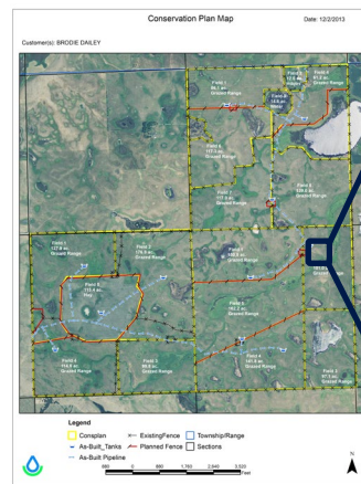
Figure 21: Map of a Deuel County, SD ranch fence and water plan resulting from an NRCS EQIP contract. Fences are permanent 4-strand barbed wire. The water system consists of underground rural water lines piped to permanent tire tanks set in concrete (upper right). Pipe trench scars are prevalent for several years after installation and may require special consideration for invasive species management (lower right). Map courtesy of Deuel County, SD Natural Resources Conservation Service, photos by Pete Bauman.
