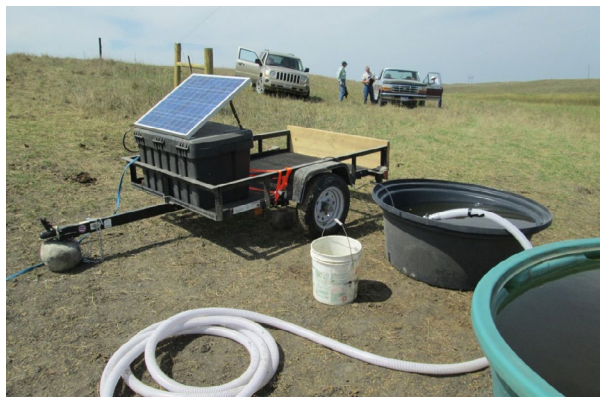
Figure 9: Photo at left shows a compact solar panel and weather resistant component system (black box) permanently mounted on a small utility trailer. The box houses a backup battery, electrical system, and supplies. Trailer space allows for transportation of tank, pump, and hose. The system at right is a commercial system with a similar solar panel and weather resistant component box mounted above a steel water tank. This system utilized a tank transport skid that is easily removed. In both cases, managers are afforded convenience and flexibility when moving livestock between pastures and water sources. Photos by Pete Bauman
