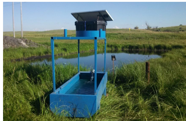
Figure 9: Photo at left shows a compact solar panel and weather resistant component system (black box) permanently mounted on a small utility trailer. The box houses a backup battery, electrical system, and supplies. Trailer space allows for transportation of tank, pump, and hose. The system at right is a commercial system with a similar solar panel and weather resistant component box mounted above a steel water tank. This system utilized a tank transport skid that is easily removed. In both cases, managers are afforded convenience and flexibility when moving livestock between pastures and water sources. Photos by Pete Bauman
