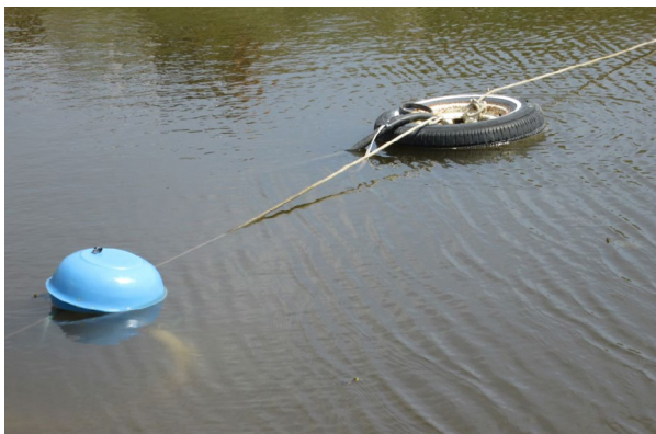
Figure 7: Example of a typical float pump installed in a dugout where cattle are excluded (top). Photo on the bottom shows a float pump (blue pump) compared to a casing pump connected to a floating tire and rim. In shallow water sources, vertical casing pumps can contact the bottom if not installed properly. Photos by Pete Bauman.
