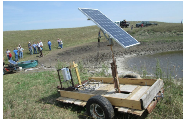
Figure 8: Photo on the top shows a permanently mounted panel system wired to a submerged casing pump. Photo on the bottom illustrates producer innovation, mounting a large panel on a homemade trailer allowing the panel to be used in several locations throughout the pasture. Photos by Pete Bauman.
