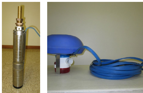
Figure 6: Example of casing pump (left) and float pump (right). Photos by Pete Bauman.
