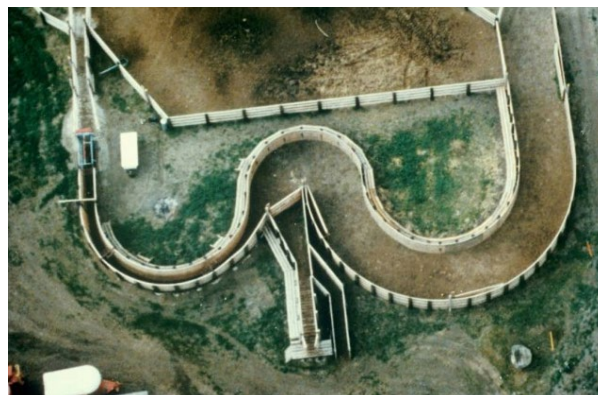
Figure 7: Aerial view of a curved alleyway and tub system. Dr. Temple Grandin. http://www.grandinlivestockhandlingsystems.com
