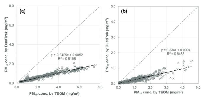
Figure 2. Comparison of TEOM versus DustTrak readings in (a) a broiler house and (b) a layer breeding house.
