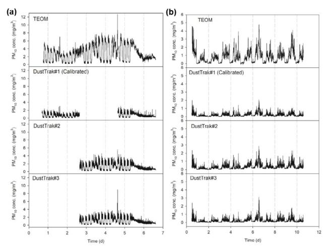
**Figure 1.** PM10 concentrations measured by TEOM and DustTrak meters in (a) a broiler house and (b) a layer breading house.
