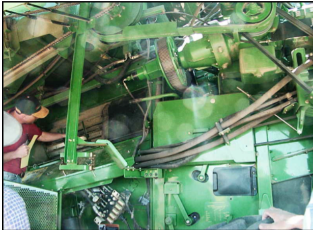
Figure 28.1. Examining the concave area and the cleaning shoe in a rotary combine during the wheat harvest.
