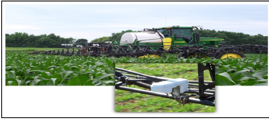
Figure 15.5. Sprayer mounted Greenseeker sensors (RT100, RT200-N, RT200-FmX). (Source: Jim Logg, Trimble.com , 2011)
