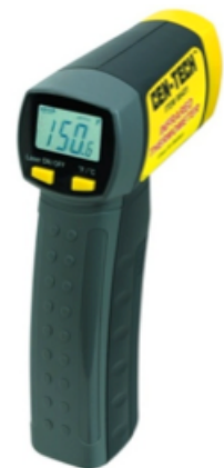
Figure 39.4. An example of an inexpensive infrared thermometer. These devices have a laser pointer and can quickly perform non-contact measurements of surface temperatures of bearings and mechanical components. (Source: www.harborfreight.com )
