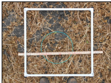
Figure 38.1. Harvest losses can be determined using a hoop or box. The green wire hoop encloses one square foot. The PVC frame encloses five square feet. For PVC frames, put a bungee cord through its ends which will allow it to collapsed and stored compactly. (Photo courtesy of D. Humburg, SDSU)
