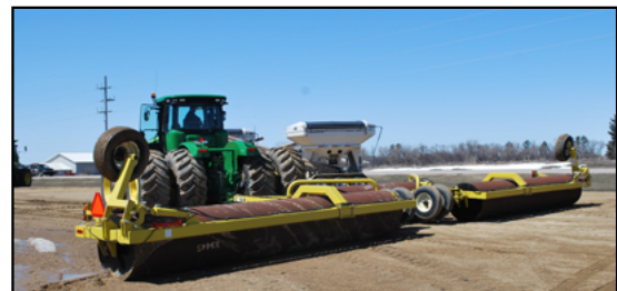
Figure 12.1. Land rollers are commonly used in preparing the seedbed in soybean production. (Photo courtesy of Schuneman Equipment Co., Brookings, S.D., and SDSU)
