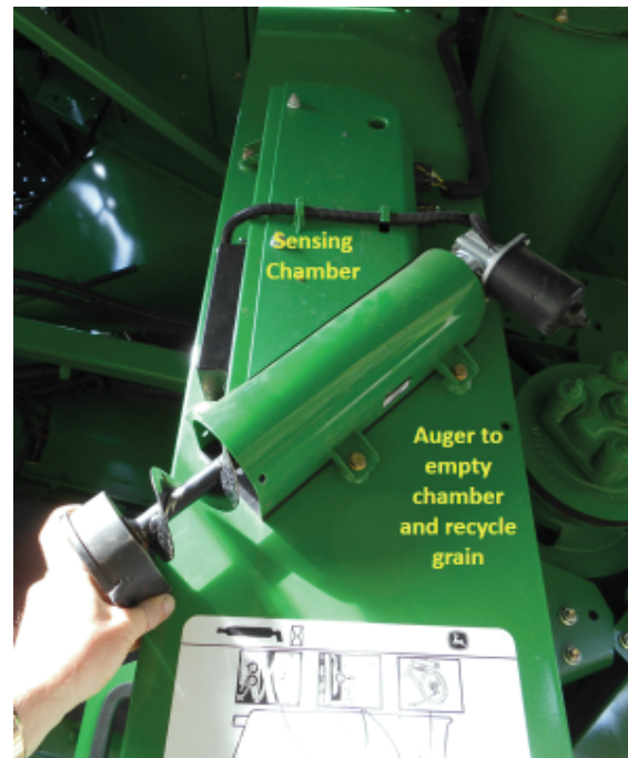
Figure 50.2 Moisture sensor sampling system on the side of the clean grain elevator. The small auger periodically empties the chamber, which refills from the clean grain elevator to take another sample. (Courtesy of authors)
