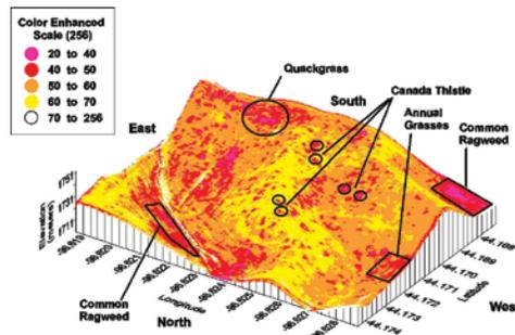
Figure 19.3 The use of remote sensing superimposed on topography map to identify area that needed to be scouted. Remote-sensing layer is near infrared (NIR) band taken from airplane in 1997. Weed patches were identified by field scouting. (Courtesy: SDSU)
