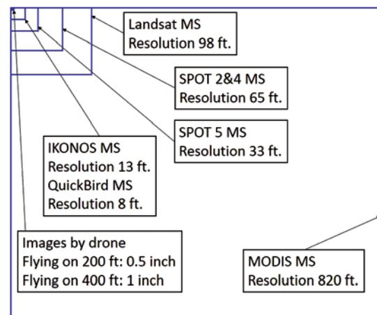
Figure 19.4 Different resolutions that can be collected by different sensors. (Dalsted et al., 2003)
