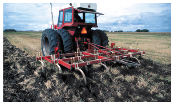
Figure 11.2 Chisel plowing wheat stubble. (Photo courtesy of USDA-NRCS)
