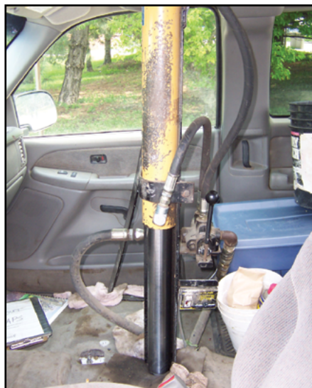
Figure 3. In-cab truck mount hydraulic probe.
